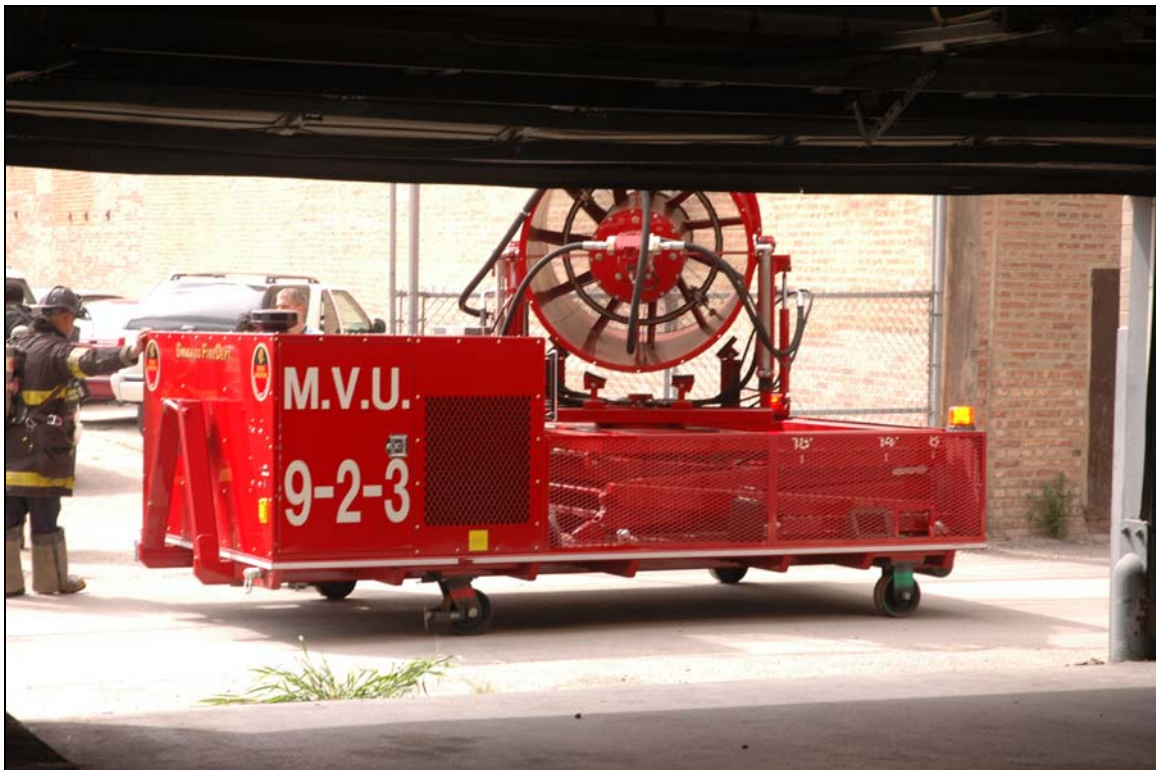
Mobile Ventilation Unit Venting Through Groud Level Garage Entrance
