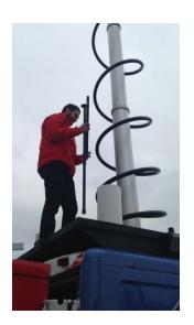
**Step One:** Apply enough air to raise the mast approximately 1.5 to 2 sections. Note that often times the largest section raises first. Following all workplace safety laws, gain access to the roof of the vehicle, assemble the piping and insert between the roof bracket and the equipment mounting bracket. See photos below.
