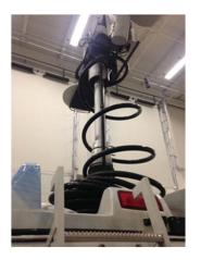
**Step Three:** With air inside the tower you should now be able to move the tower sections up and down as needed to expose the sections one at a time, starting with the smallest (topmost) section. Refer to Step 4 for cleaning instructions. Please note as you move to the larger sections it will be necessary to add a little bit of air to keep the larger tubes from retracting back inside the larger sections.
