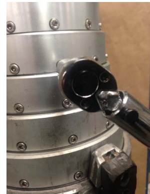
Tighten to 31.86 inch pounds using Torque Wrench
