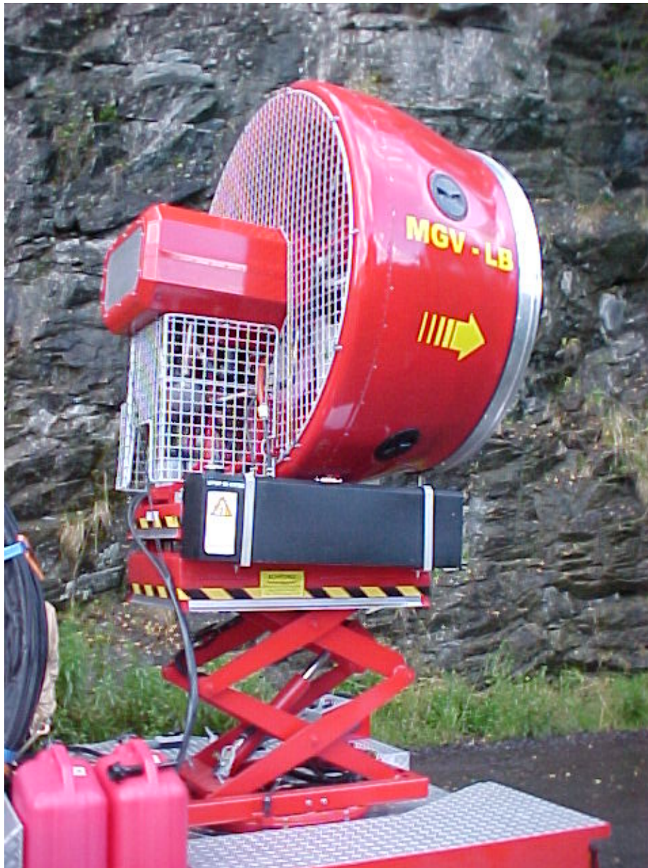
Truck mounted MVU elevated in preparation for conducting PPV.
