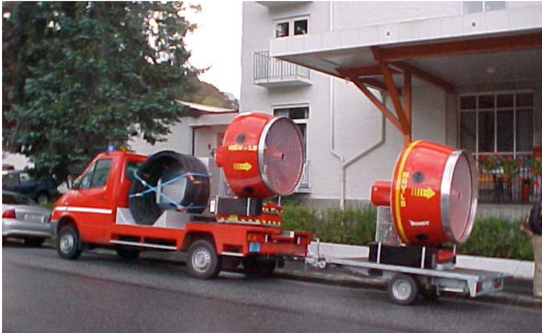
One truck mounted and one trailer mounted MVU were used for the test.
