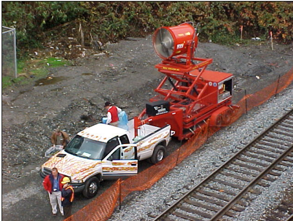
Figure 2: 48" Trailer Mounted MVU Used for Test
