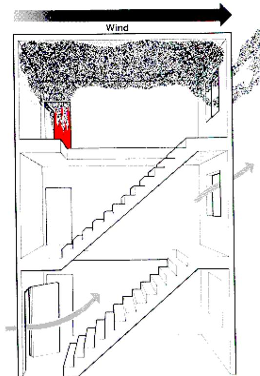
*Fig 3:Improving Firefighter's access using defensive ventilation*
