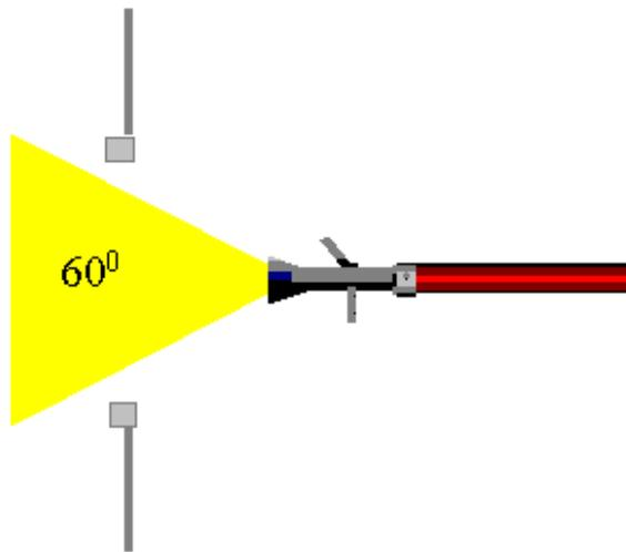
*Fig 4: Ventilation using a branch*
