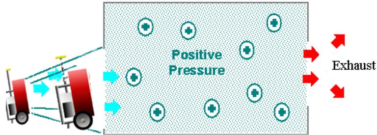
*Fig 7: Using two fans inline*
