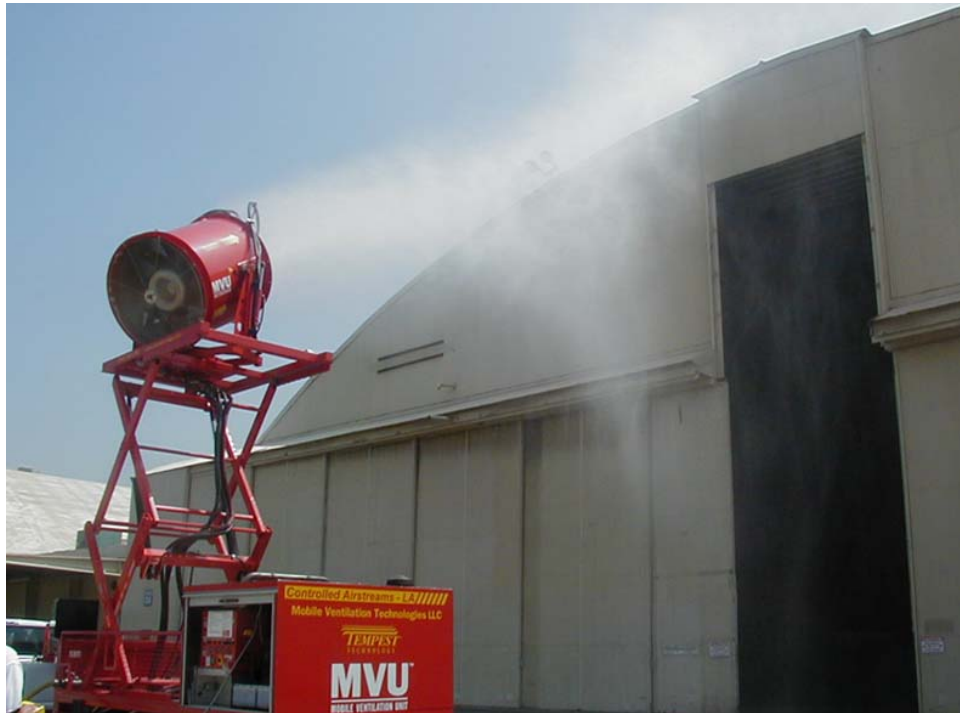
MVU Misting System for Cooling and Knockdown of Suspended Gases
