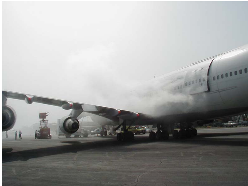
MVU Exhausting Smoke Through Rear Cargo Door of 747
