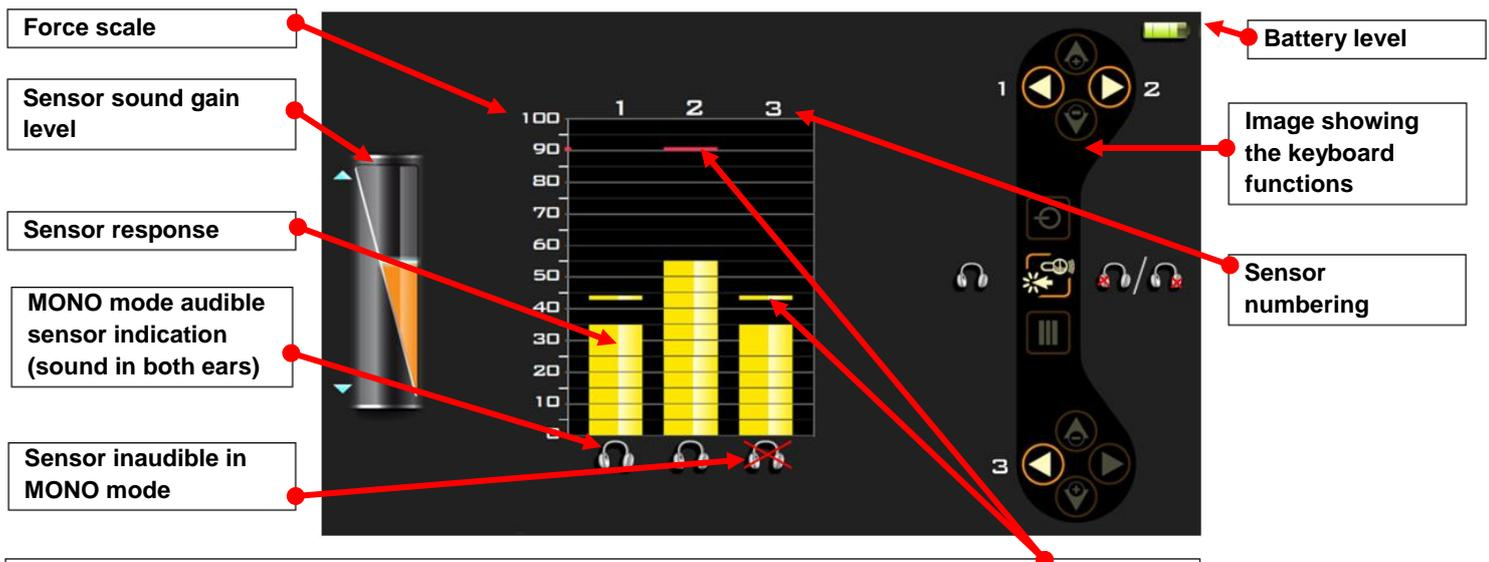
The yellow marker shows the sensor's maximum response. The marker turns red on the sensor that detects the highest peak. If both sensors detect the highest peak at the same time, then they will both be red. This marker is carried over onto the scale for easier readings.
