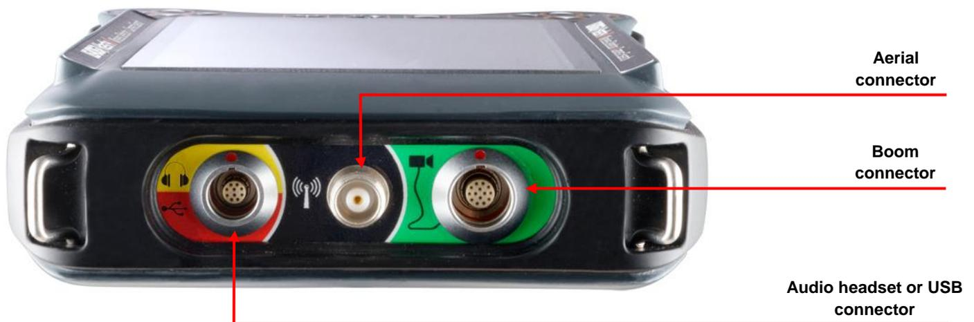
The audio / USB connector is used to connect either the audio headset or a specific USB stick supplied by **LEADER** to update the software when necessary. No other USB peripherals should be connected.
