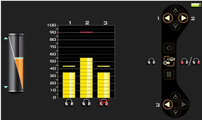
The "**seismic**" mode can be selected when one or more seismic sensors are connected. Here three sensors are connected.
