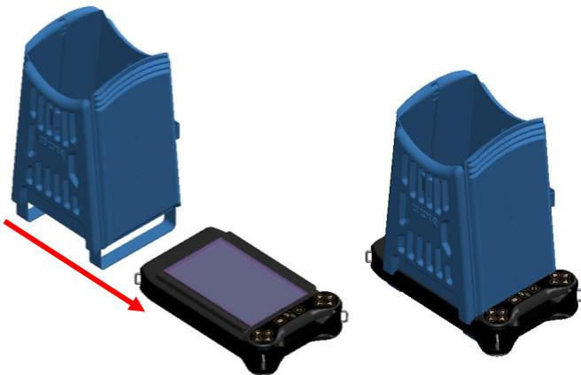
It is stored flat for easier transport. An elastic on its side is used to keep it flat and fix it to the control box. By placing it on the screen face, it protects the screen when moving around when the search device is not in use.
