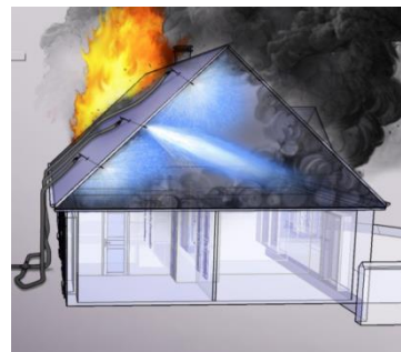
Establishment of a firewall when the fire has gone through the roof
