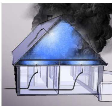
Extinguishing a fire in a multi-layer roof or in false ceilings
