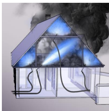
Extinguishing a fire under roof spaces: attack all compartments on fire
