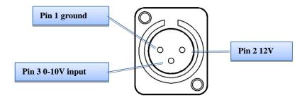
The input signal at pin 3 will trigger the machine operation when it is taken above 2V.
