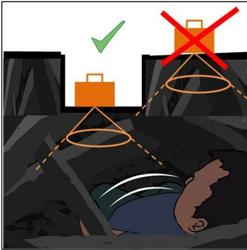
The compact size of the UWB sensor allows it to be inserted into cavities and gain several centimetres to increase the percentage success of detecting a victim.
