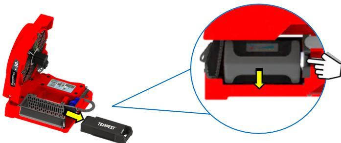
Ensure that the fan is switched off before disconnecting the battery.
