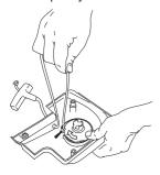
CAUTION! Check that the pulley can be turned an additional 1/2 turn when the starter cord is pulled all the way out.
