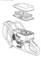
If the machine is low on power, difficult to start or runs poorly at idle speed: always check the spark plug first before taking any further action. If the spark plug is dirty, clean it and check that the electrode gap is 0.020 inch (0.5 mm). The spark plug should be replaced after about a month in operation or earlier if necessary.
