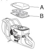
Remove the foam plastic filter. Wash the filter well in tepid soapy water. After cleaning, rinse the filter well in clean water. Squeeze out and allow the filter to dry. NOTE! High pressure compressed air can damage the foam.
