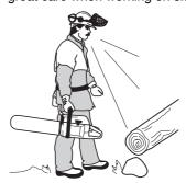
Take great care when cutting a tree that is under tension. A tree that is under tension may spring back to its normal position before or after being cut. If you position yourself incorrectly or make the cut in the wrong place the tree may hit you or the machine and cause you to lose control. Both situations can cause serious personal injury.
