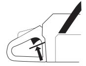
• Press the throttle lock and make sure it returns to its original position when you release it.
