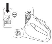
The engine is stopped by pushing the stop switch to the stop position.
