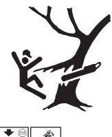
6 Before moving your chain saw switch off the engine and lock the chain using the chain brake. Carry the chain saw with the bar and chain pointing backwards. Fit a guard to the bar before transporting the chain saw or carrying it for any distance.
