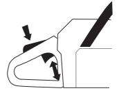
Start the chain saw and apply full throttle. Release the throttle control and check that the chain stops and remains stationary. If the chain rotates when the throttle control is in the idle position you should check the carburetor idle adjustment.
