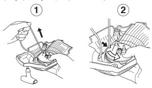
Undo the screw in the centre of the pulley and remove the pulley. Insert and fasten a new starter cord to the pulley. Wind approx. 3 turns of the starter cord onto the pulley. Connect the pulley to the recoil spring so that the end of the spring engages in the pulley. Fit the screw in the center of the pulley. Insert the starter cord through the hole in the starter housing and the starter handle. Make a secure knot in the end of the starter cord.
